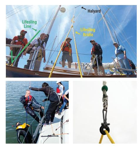
one pointing up and the other down since the lifesling can float either side up. Have a crew with a searchlight light up the rope and lifesling as his *only* duty.
